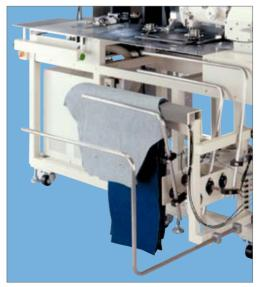
The stacker provides a capacity of 64 pieces of finished products. In addition, the stacker is equipped as standard with a stacker-capacity detector.
