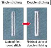
• For double stitching, the bartacking section is skipped and only the parallel sections are sewn twice. This prevents any excessively tight finishes in the bartacking section of the buttonhole. • First- and second-round stitches can be
