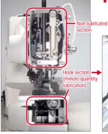
• Only a minute-quantity of clean oil is fed to the hook section from the oil tank.
