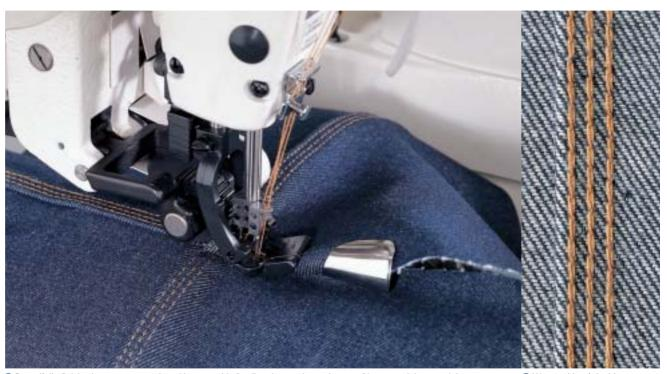
Beautifully-finished seams are produced by smoothly feeding the overlapped parts of heavy-weight material.
