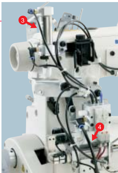
3 Presser lifter drive mechanism air cylinder 4 Thread trimmer drive mechanism air cylinder
